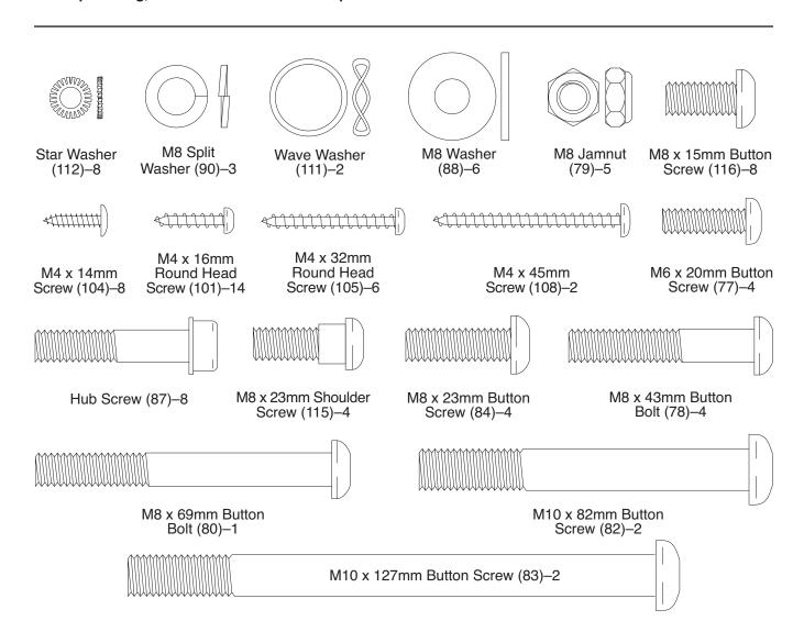
1. While another person lifts the Base (1), attach the Front Stabilizer (6) to the Base with two M10 x 82mm Button Screws (82).
